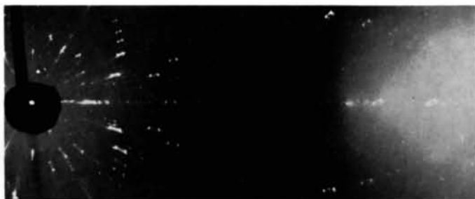
Fig. 12. Laue photograph of the upper part of crystal 6. Polytype 6R ; conditions as in Fig. 4.
