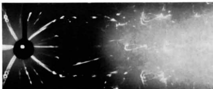
Fig. 11. Laue photograph of the lower part of crystal 5. Mixture of 6R and other unidentified polytypes; conditions as in Fig. 4.
