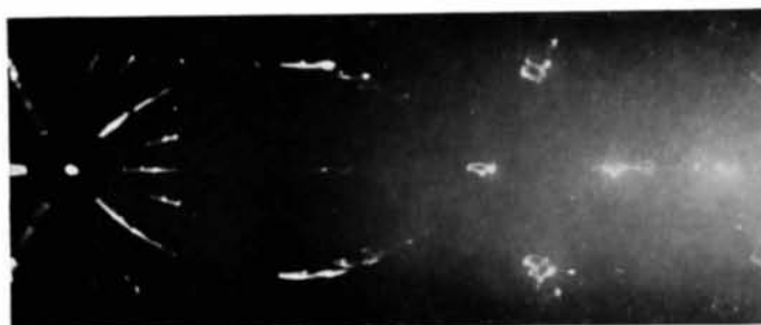
Fig.10. Laue photograph of the upper part of crystal 4. Polytype 6R; conditions as in Fig.4.
