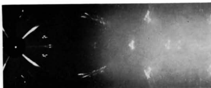
Fig.8. Laue photograph of the lower part of crystal 3. Mixture of 6R and other unidentified polytypes; conditions as in Fig.4.
